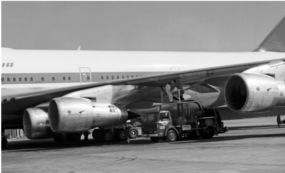
No 1 - 747-238 VH-EBA – Pratt & Whitney JT9D-3A Fifth Pod Installation
