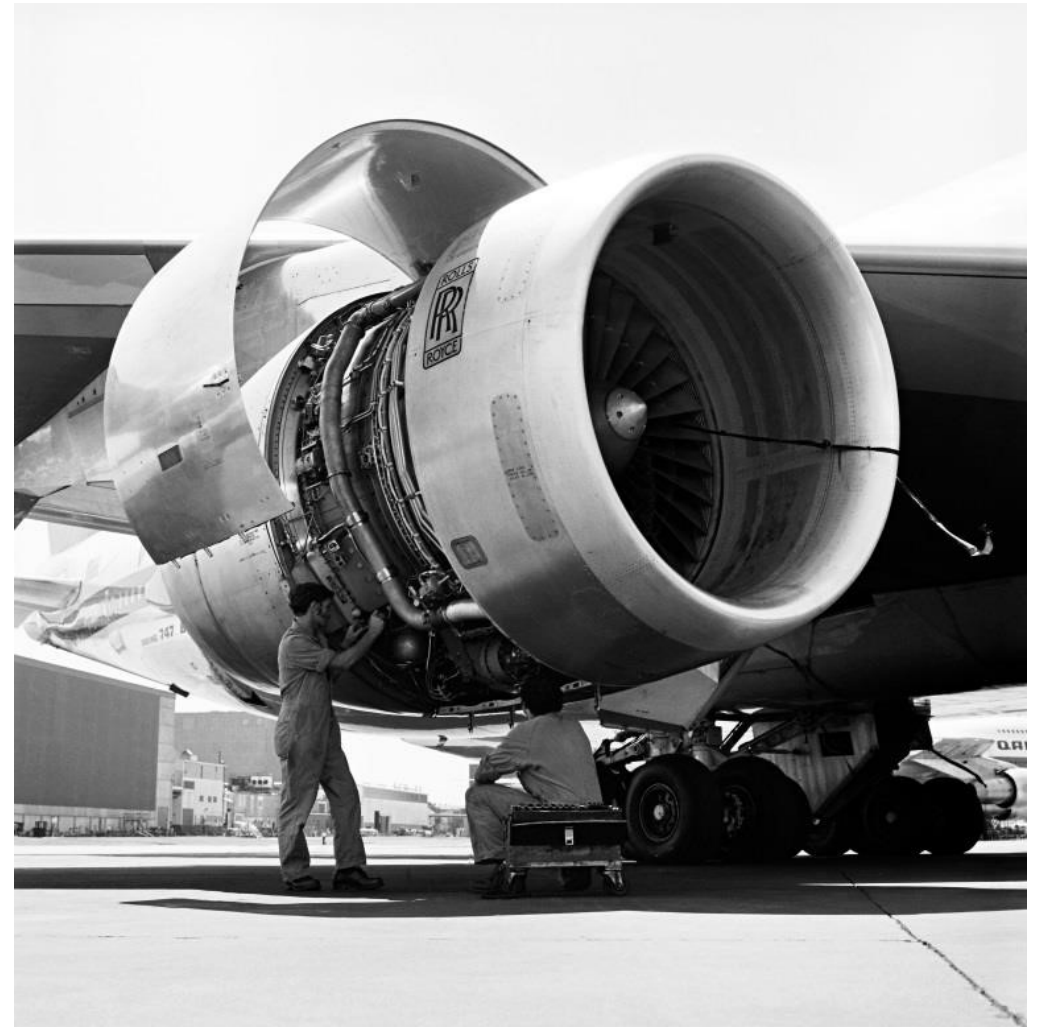
No 22 - 747-38SP VH-EAA – Rolls Royce RB211-524B2 Engine
