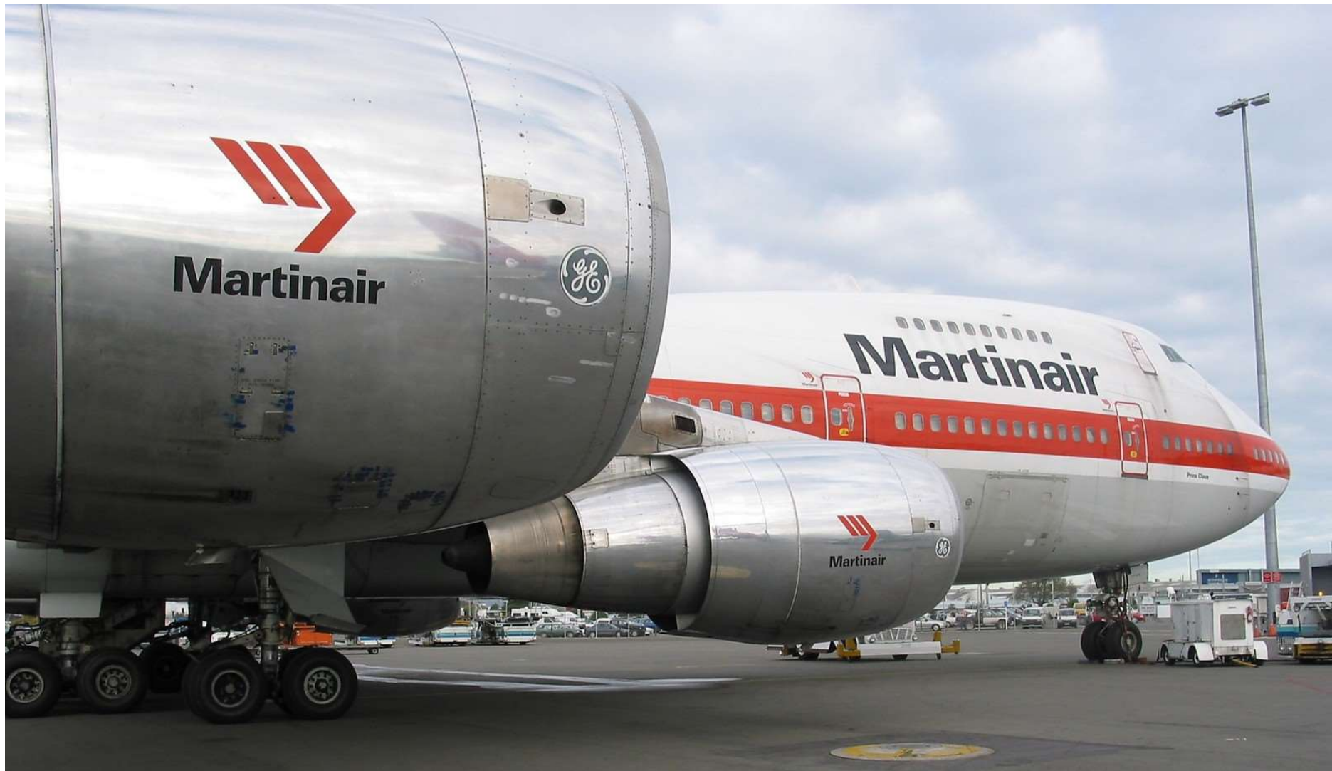
No 34 - 747-21A PH-MCF – General Electric CF6-50C2 Engines
