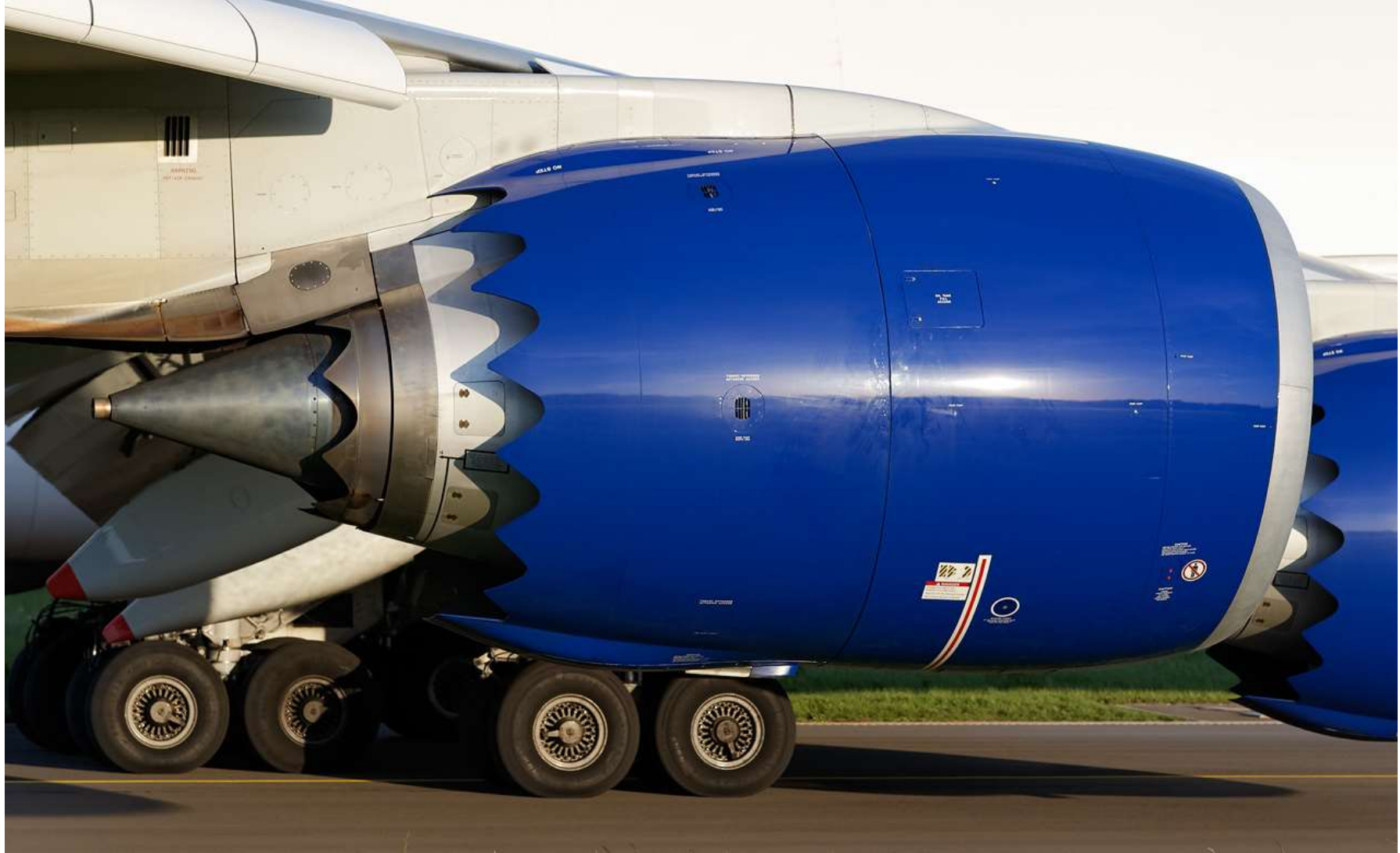
747-87UF Freighter – General Electric GEnx-2B Engines
