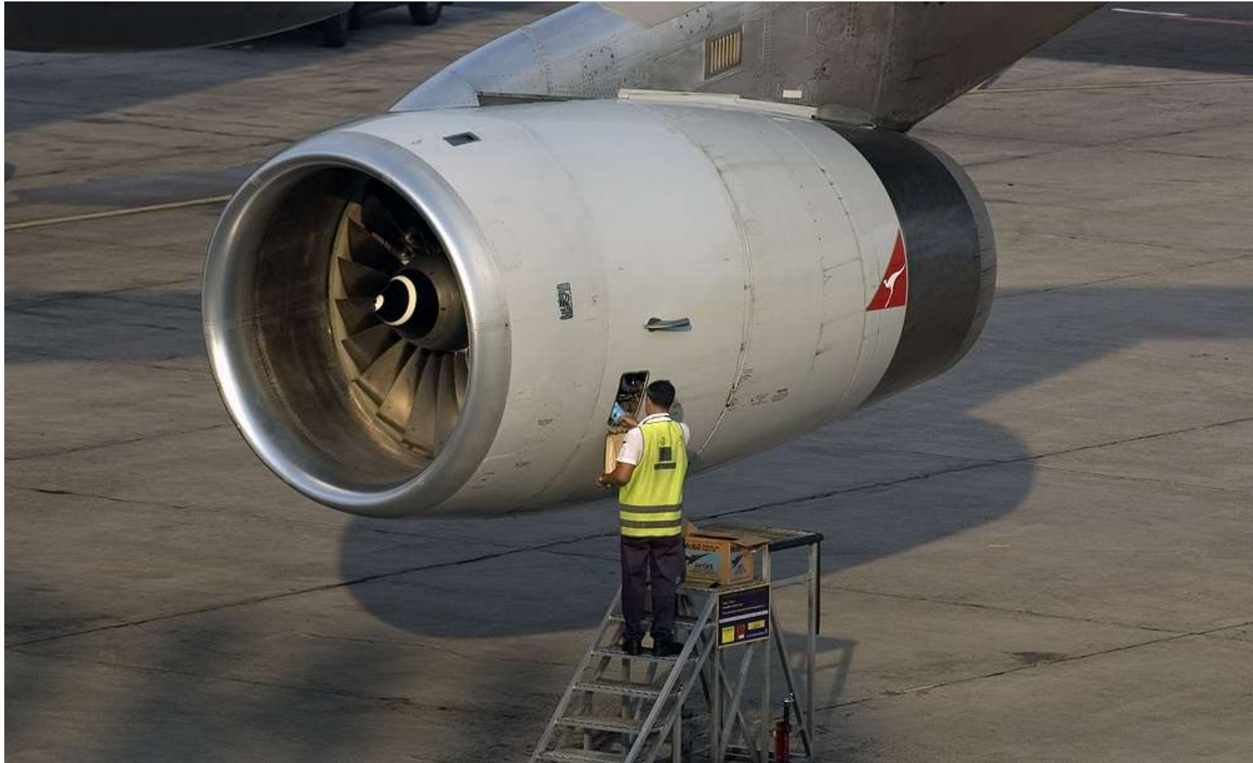
No 35 - 747-438 VH-OJA – Rolls Royce RB211-524G2 Engine
